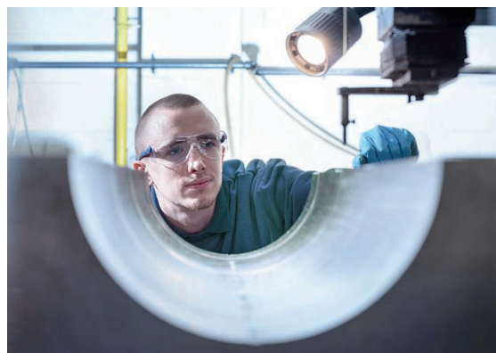
An engineer uses a technique known as electrical discharge machining to drill holes in a metal part.
